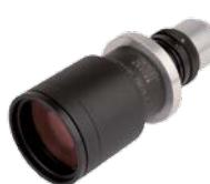
The series Correctal® T Compact has a very short working distance and a short length. All lenses have a C-mount thread and a variable iris. Lenses of this series are available with coaxial illumination as well. The clear aperture is 60 mm. The lenses are suitable for sensors with a minimum pixel size of 4.6 µm.
