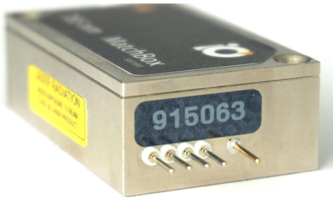
Figure 1-2. Serial number is marked on the back of the laser body, right above the connecting pins.
